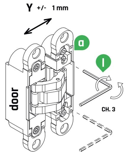
**Adjusting the Y axis - door panel in/out**
