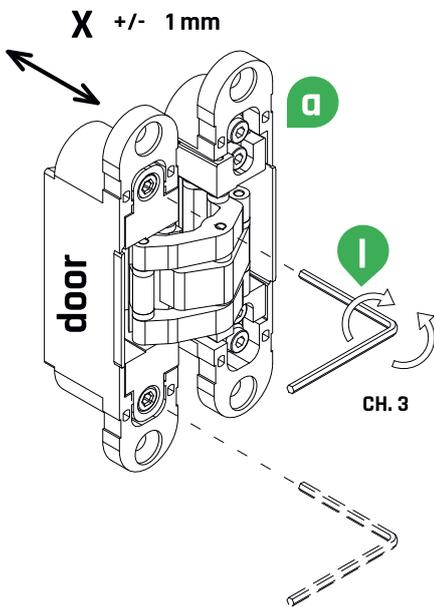
**Adjusting the X axis - door panel right/left**
