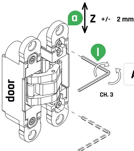
**Adjusting the Z axis - door panel up/down**
